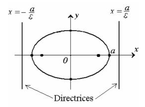
3) For any point of ellipse (3), the ratio of the focal distance to the distance from the corresponding directrix is equal to the eccentricity of the ellipse:
