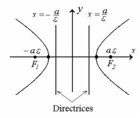
3) For any point of hyperbola (8) the ratio of the focal distance to the distance from the corresponding directrix is equal to the eccentricity of the hyperbola.
