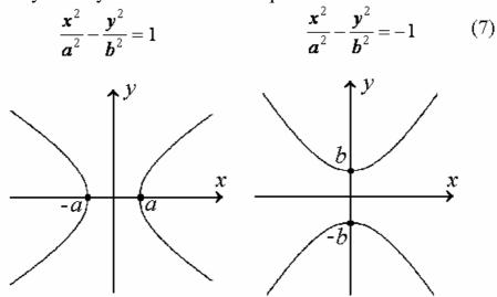
Equations (7) are called the **canonical equations of a hyperbola**. The corresponding coordinate system is said to be the canonical system. In this coordinate system, the coordinate axes are axes of symmetry, that is, if a point (x, y) belongs to the hyperbola then the points (-x, y), (x, -y) and (-x, -y) also belong to the hyperbola.
