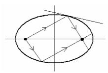
In other words, at any point of an ellipse, the tangent line forms equal angles with the focal radiuses.
