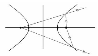
The drawing illustrates that reflected rays form a divergent beam.
