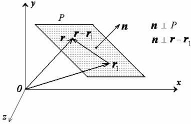
Thus, equation (3) describes a plane that passes through the point  $M_1(x_1, y_1, z_1)$ . The coefficients A, B and C can be interpreted as the coordinates of a normal vector to the plane.
