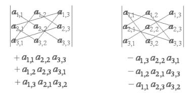
The elements on a diagonal or at the vertices of a triangular form the product of three elements. If the base of the triangle is parallel to the leading diagonal of the matrix, the product keeps the sign; otherwise, the product changes the sign.
