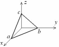
Equation (6) is called the equation of a plane in the intercept form. For instance, the equation
